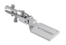
This mouse adaptor holds the mouse head by means of a palate bar and nose clamp without ear bars. If offers vertical requisition to make the head level or at a certain angle. The skull of mice and neonatal rats is relatively thinner than that of an adult animal, so that the use of ear bars can deform the skull and effect the animals breathing. But this way of holding the animals head without bars compromises the stability and therewith requires more experience of the operator.
