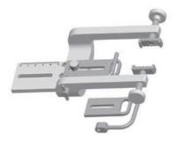
This adaptor holds the rabbits head through a dedicated cheekbone clamp, nose clip and an adjustable incisors buckle. The distance between the two cheekbone clamps can be precisely adjusted by a screw knob. An infant and an adult buckle is included. The adjustable range for the adult incisor buckle is 43,5mm, and the range for the infant one is 26,5mm. The horizontal range for the adaptor plate is 40mm.
