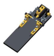
For PET/CT brain imaging of animals, it is difficult to hold the head firm and stable, while keeping the animal under anesthesia. Based on PET/CT imaging requirements, a special adaptor was developed for holding the head of tree screws firm and stable with high quality non-metallic materials. Also this adaptor has a gas mask to anesthetize the animal while imaging. The Tree shrews can wake up in 2-5 minutes after the experiment.
