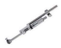
In electrophysiological stimulation or recording experiments, it requires critical accurate electrode manipulation. This microdriver will improve operational accuracy in the vertical direction to  $10\mu m$ . It is easy to handle and various electrode holders are available to work with the microdriver.
