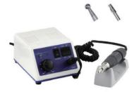
The high speed drill is designed for opening the skull in stereotaxic surgery, to implant electrodes, canula, microdialysis probes, etc. This Drill is easy to handle and operate.
