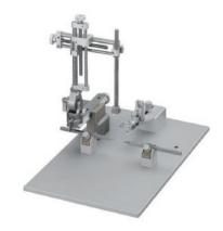
This portable / rail rat Stereotaxic Instrument, using blocks instead of the traditional U-shape frame, provides a spacious, open operating space for researchers.
