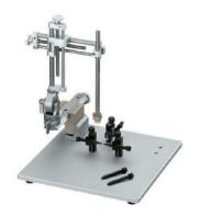
Designed to use adaptor blocks to replace the traditional U-frame assembly. It holds the mouse or neonatal rat firmly and accurately. This instrument provides easy access to the animal and offers an open work area.
