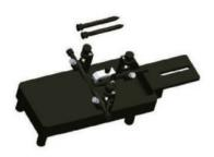
This adaptor is similar to the mouse adaptor 68U030 and it can be fixed on the U-frame Stereotaxic Instruments. It is not necessary to add accessories to elevate the animals body once the head is firmly held which simplifies tedious operation while keeping the rat breathing well, incisor, nose clip and the ears bars can be adjusted up and down within 20mm range, which makes it easy to adjust the level of the rat brain.
