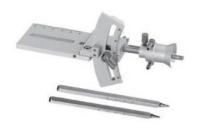
This design integrates the gas anesthesia mask function while holding the rats head firmly. The adaptor can rotate the head to multi-angels without blocking the anesthetic gas delivery. The Dorsal/Ventral adjustment rage is  $40^{\circ}$  (+ $20^{\circ}$  ~ - $20^{\circ}$ ) with  $1^{\circ}$  accuracy. The horizontal adjustment range is 43,5mm, and the diameter of the inlet/outlet of gas anesthesia mask is 2mm.
