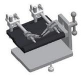
This spinal adaptor can apply for mouse study. During the experiment, the mice can be lifted to avoid breathing effect. This adaptor can be rotated with different angles, depending on the height of the base, to facilitate observation under a microscope. Also, the base plate can be easily fixed to the microscope stage by T-shape screws.
