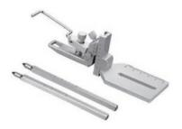
This adaptor holds the head through the 45° ear bars, incisor and nose clamp. To hold guinea pigs with different weight, the nose clamp has 30mm adjustable range along a vertical dovetail slide and 50mm adjustable range in horizontal direction.
