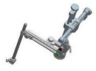
A/P slide attachement can be easily installed on the operating arm of the V-shaped groove, and the sliding range is 60mm, with 0,1mm accuracy. When the electrode of probe is held perpendicular to the Z-axis, it can be manipulated in the horizontal direction, which provides fine control for targeting the coordinated of the brain atlas location.
