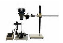
The standard microscope set-up is with the 0,3x objective (ABCD) is designed for use with a stereotaxic instruments because of the 276mm working distance. It can also be used for microsurgery.
