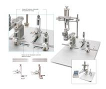
This portable rat and mouse Stereotaxic Instrument (model 68U526) is a complete set and is also available as digital model (model 68U528).
