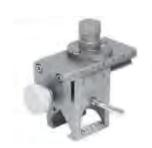
This microdriver can be fine-tuned in the range of 25mm with  $50\mu m$  steps. It makes the moving of manipulators more accurate on the rail of MRI compatible/ large animal or rail mounted stereotaxic instruments.
